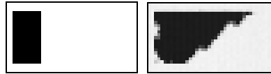
Fig. 6: The input & initial state and snapshot of the output pattern if the coupling is positive. (Chip measurement)
