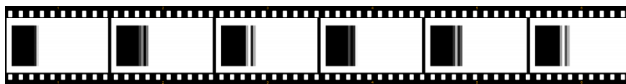
Fig. 4: The time evolution for Template 1, snapshots of the state. Observe that the propagation decays spatially after a few pixels, but the oscillation remains. The initial state is the same as the input. (Simulated results, size: 41 \times 23 )
